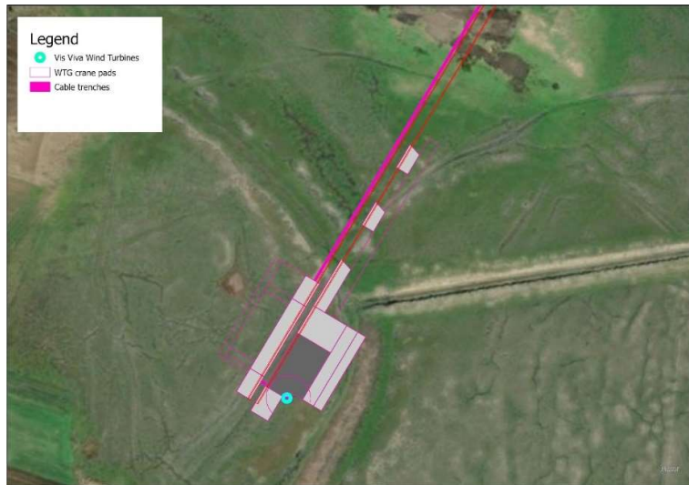
Figure 2-3 Typical WTG and Associated Working Platforms
