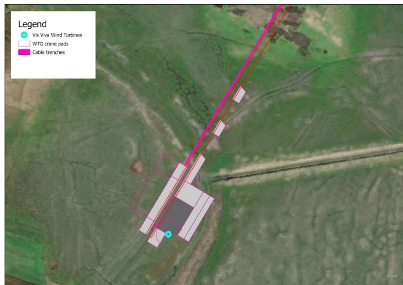
Figure 2-3 Typical wind turbine site and its paved areas
