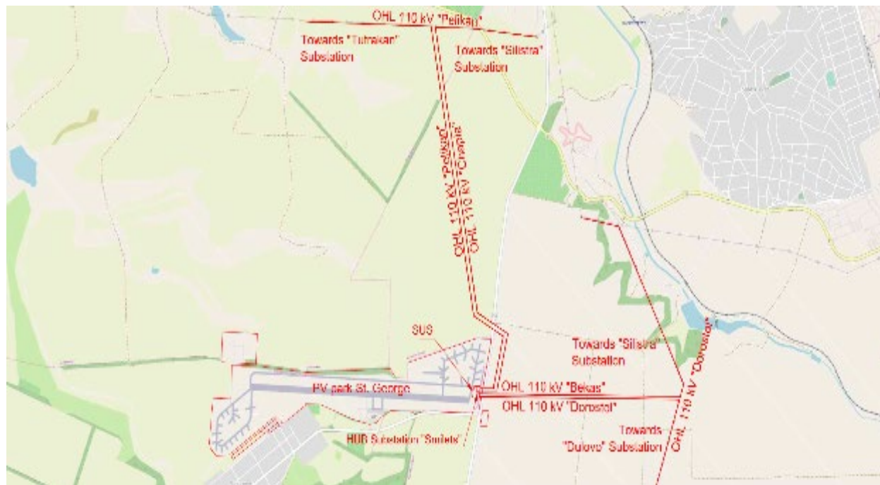
Figure 17: St. George substation sites and PV substation and indicative routes of “Pelikan” and “Dorostol” 110kV OHTL interruption points
