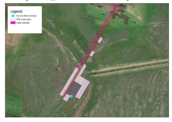
Figure 2-3 Typical WTG and Associated Working Platforms
