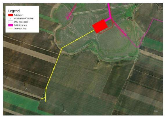
Figure 2-4 Transformer Station Location and OHL Connection to the 400kV OHL Cernavoda - Stâlpu Line
